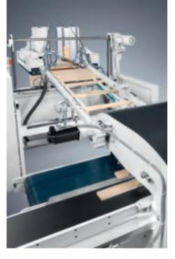
For the clear identification of the pieces after the cutting, inkjet or label printers are used.
