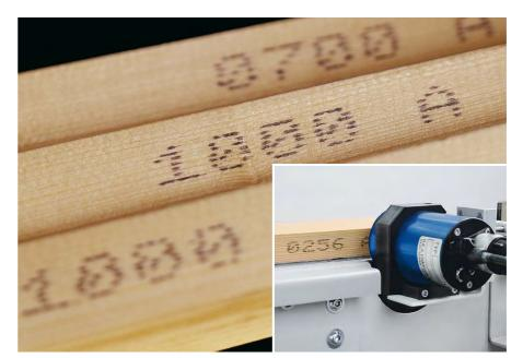
Easy handling of the sawn timber, warehouse identification, order-based assignment, product-based logistics – in all these cases, the identification of the cut lengths has an important role to play. Thus, a clearer overview, lower costs or in general the use of cost-optimised production processes are made possible. Number or code labelling is performed directly on the workpiece, from the side or above.
