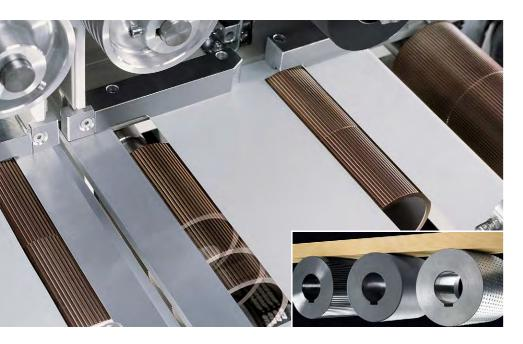
Different wood qualities impose different requirements. Thus, the feed rollers of the OptiCut 200 can be changed very quickly in order to respond to the respective requirements. Rough and planed qualities can now be readily processed in the same shift, and resincoated rollers are easily cleaned for consistently high performance in every shift.
